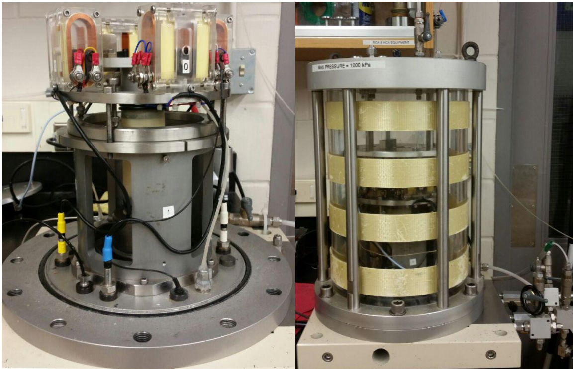
Figure 3.7. Left: Drive system on top of the sample. Right: Assembled resonant column apparatus.
