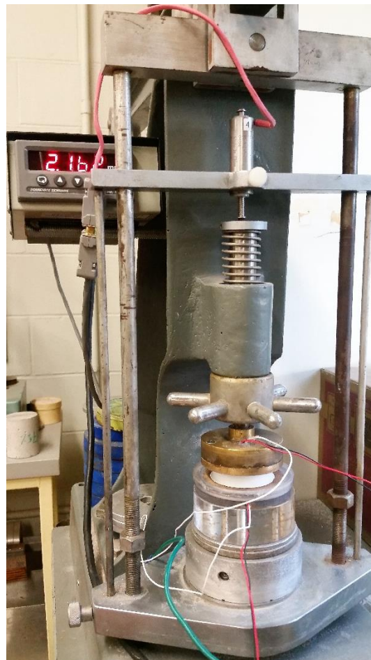
Figure 3.6. Piezoelectric ring actuator incorporated in an oedometer. A LVDT is used to track changes in sample's height.
