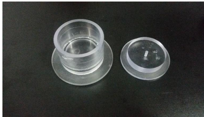
Figure 3.2. Typical LEXAN mold for preparation of mini-puck PVA-C samples.
